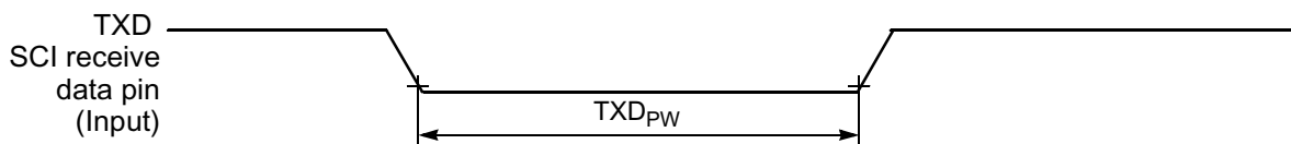
Figure 10-16 TXD Pulse Width
