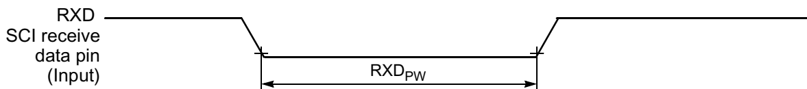
Figure 10-15 RXD Pulse Width
